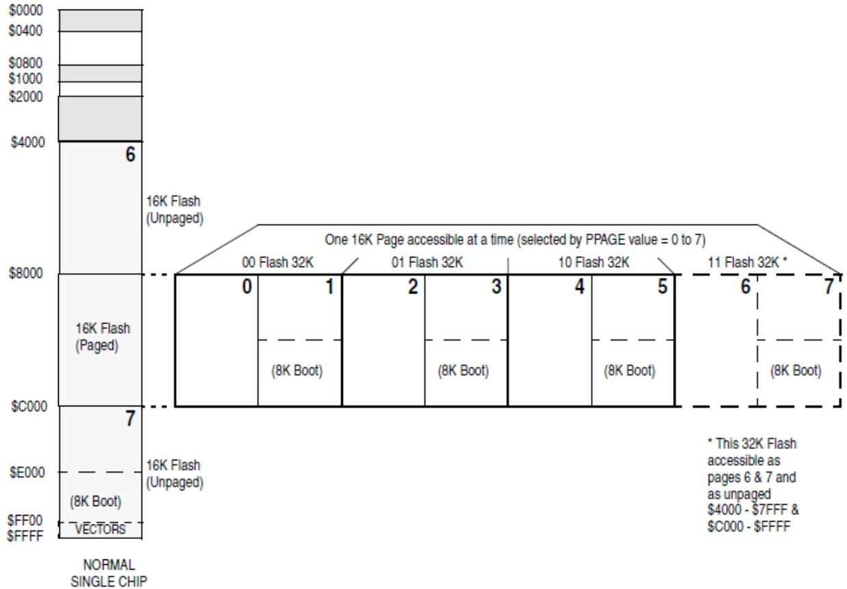
This means that the whole Flash memory, with a size of 128KB, is split into 8 different pages of 16KB each. The access to each page is done by setting which one is used before operating on it.
